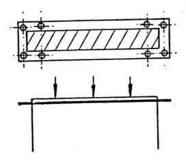
Therefore, header plates must be designed with overhang to permit the header plate to diaphragm.
